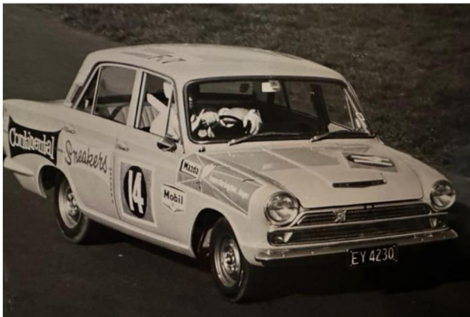
***Ford Cortina 1200 c.c. three bearing crankshaft as raced by Rodger Anderson and Kevin Masterson at Pukekohe with Rodger Anderson at the wheel. Note the 'cool' column change gear lever hand ready to 'hook another cog'.***
